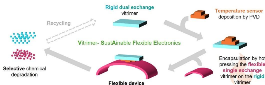
Figure 1: Lifecycle of a temperature sensor deposited on a rigid vitrimer and protected by a flexible vitrimer (applied by hot-pressing), with differences in the chemistry of the two vitrimers enabling selective chemical degradation.
